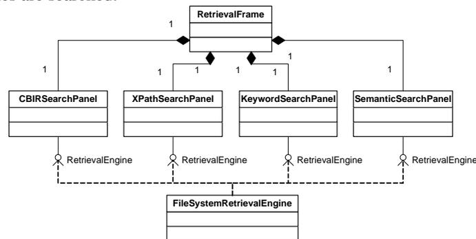
Fig. 5. Simplified UML diagram of the Emir retrieval architecture
